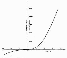
Fig. 5. (b.) Carborundum Crystal Rectifier.
