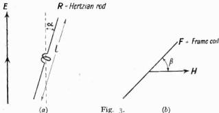
maximum value of the electromotive force induced in the aerial is  $E \cos \alpha$ . In Fig. 3 (b) F represents a plan view of a vertical loop of area "A" in the magnetic field of maximum intensity H, the plane of the loop making an angle  $\beta$  with the magnetic field. The electromotive force induced in each turn of the loop has a maximum value of  $AH2\pi n \cos \beta$ , where "n" is the frequency corresponding to the wave.
