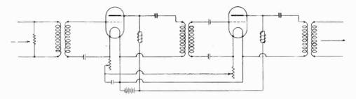
Fig. 1a. Circuit of amplifier employing tuned transformers.
