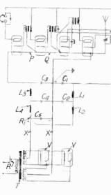
and condensers, LI CI, L2 C2, and L3 C3, L4 C4, C5. The first system is an ordinary smoothing device for the high tension supply, while the second system is for the filament supply, which is further controlled by a variable resistance RI. This second filter system contains enough resistance to lower the voltage to a suitable value for the filaments. The filaments, of course, are connected in series.
