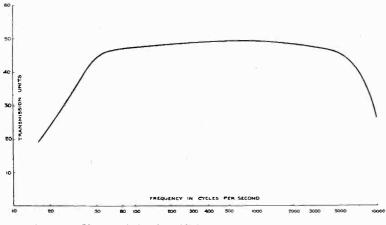
Fig. 1. Characteristic of amplifier employing tuned transformers.
