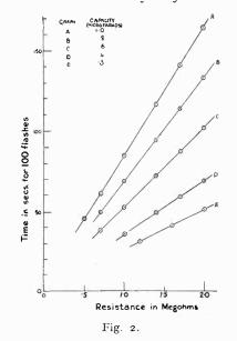
the other ractors being constant, T is a measure of R in one case and of C in the other. The application of this to the comparison of capacities and high resistances is obvious.
