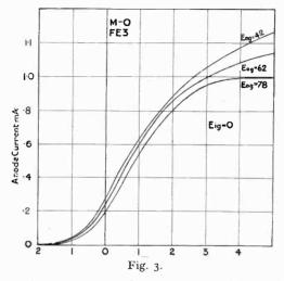
anode voltage under these conditions is rather higher than 16. From the curves we find  $\mu = 5.5$ ,  $R_a = 42000$ .
