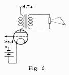
the primary of the intervalve transformer was observed even when there was no modulation of the carrier wave. This was eliminated by shunting a  $\cdot 000 2\mu$ F condenser across the winding. This  $\cdot 06$ volts thus represents an appreciable and avoidable loss.
