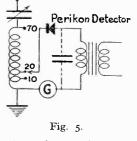
the comparative freedom from distortion being, doubtless, that the flow produces little effect on the total charge in the  $0.1 \mu F$ coupling condenser, whereas with transformer coupling it would be sufficient practically to short-circuit the secondary.
