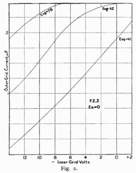
show the normal effect of increasing the IG volts—similar to more filament heat. The
