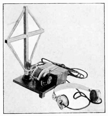
A "High-tensionless" Receiver : range 20 yards on 5XX i It is used at Chelmsford as a test set.
