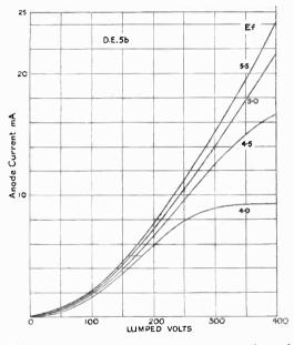
The anode impedance is seen to be of the amount usually associated with an ordinary small valve (30,000–20,000); but it is extraordinarily low in view of the  $\mu$ of over 20. The filament efficiency is of the usual order for the D.E.5 filament.
