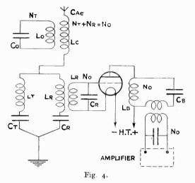
being forced from the near-by transmitter,  $N_R$  being received from the distant station. These two frequencies beat together and produce a lower frequency  $N_o$ , which can be detected and amplified without fear that the amplifier will suffer wipe out from  $N_T$ , it being adjusted only to deal with frequencies of the order of  $N_o$ , which are far removed from those of  $N_T$  or  $N_R$ .
