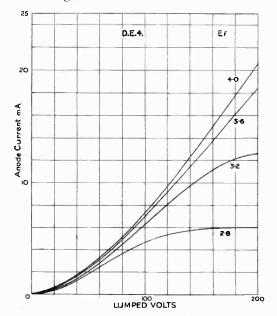
2.8, 3.2, 3.6, and 4.0V, and the results appear in the table. It will be seen that the output is fully up to that of the D.E.5, reaching 50mA at 4.0V. The anode impedance, on the other hand, is rather higher, though still very low. It falls to 9.300 ohms at 4.0V, the D.E.5 falling to 6.000 at 5.5. The  $\mu$  is similar in both valves—about 7.
