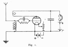
as large a voltage as possible across its inductance; and this means a large inductance. To enable a large inductance to be used, while still tuning down to the neighbourhood of 300 metres, means putting an aerial condenser in series with it. So that our typical aerial circuit uses a tuning condenser and fixed coil.
