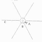
A boss B, adapted to be fixed on to an aerial wire by means of a set-screw A, carries a spike or number of spikes C, which act as discharging points to dissipate any electrostatic charge which may accumulate on the aerial. The patentee is
