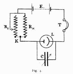
K being arranged so that either  $R_s$  the known variable resistance or  $R_x$  the unknown resistance can be introduced into the circuit at will.
