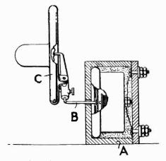
a gramophone sound-box C. Thus telephonic vibrations produced in A are reproduced in the gramophone system. (Patent No. 213,936, R. E. B. Wakefield.)
