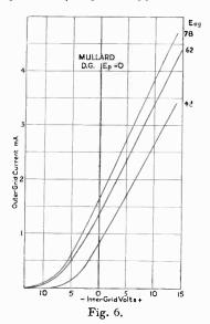
With the anode held at oV, input to IG and output from oG, the valve behaved exceedingly well, as will be seen from Fig. 6. The
