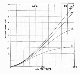
The valve was tested at 1.4, 1.6, 1.8 and 2.0V, on the filament, and its constants will be gathered from the accompanying table. The first exceptional point is the very large output, this being 10mA at the lower rated voltage, and no less than 19
