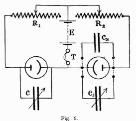
the same note is heard or the original beat frequency is obtained, when, of course, the decrease in  $C_x$  is equal to the increase in  $C_y$ . This progress can be continued until  $C_x$  is calibrated in terms of  $C_y$ . Their relation can be recorded graphically if a handy record is desired.
