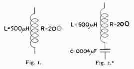
impedances, can be combined in series or parallel just as simple resistances : thus if we have several impedances  $Z_1$ ,  $Z_2$ ,  $Z_3$ , etc., all in series, the total impedance Z is given by
