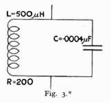
resistance of 20O; as we should expect, the condenser has partly neutralised the inductance.
