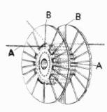
are separated by string in order to provide an air space between them. A former for use in constructing the coil is shown in the drawing.
