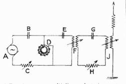
and D a frequency multiplier such as is common in long-wave high-power stations. Condenser E and transformer 6 form a system resonant to the desired frequency which serves to transfer the output of D at this frequency to the intermediate circuit and aerial system. We do not quite see where the novelty lies, however, in the mere use of an intermediate circuit.
