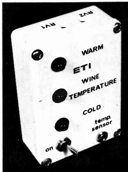
Above, the complete unit while below the sensor, a bicycle clip painted black with the sensor epoxied to it.
