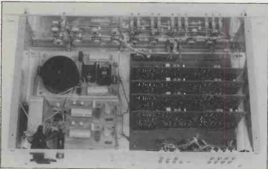
External and internal views of a custom-built synth unit employing four Voice Cards in its design.
