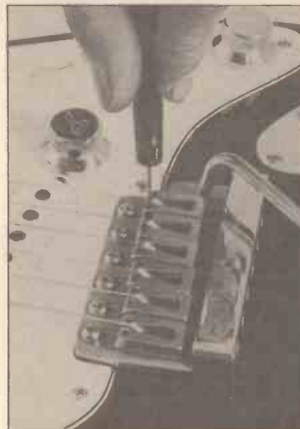
Action adjustment using Allen key.
