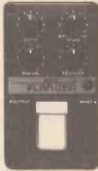
FLANGER FL-01 Function: Speed, Depth, Feedback, Manual
