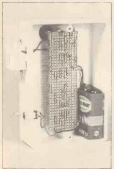
Rear view of unit showing Veroboard, buzzer, etc. in position.
