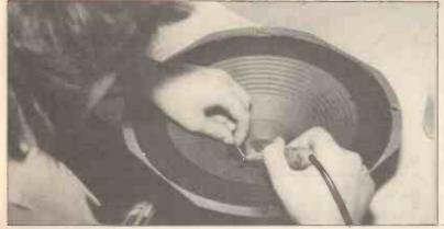
Soldering wire connections to cone.
