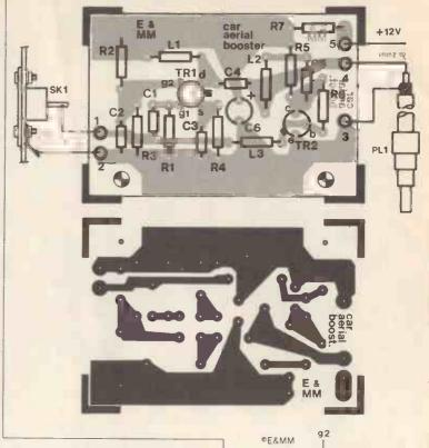
off-board connections, the board can be mounted in the case prior to making the connections to SK1, the output lead, and the positive supply lead. If a metal case is used, fit spacers over the mounting bolts so that the connections on the underside of the board do not short-circuit to the case. It is then only necessary to fit a car aerial plug to the output lead and the booster is ready for installation and use.
