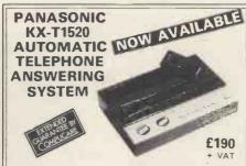
One of the most technically advanced telephone answering units available, the KX-T1520 features a double cassette system, a C60 cassette for incoming calls, which can be limited to 30 secs each or recorded in their entirety, and a 20 sec continuous loop cassette for your outgoing messages which are recorded through the built-in microphone. Your telephone conversations can also be
