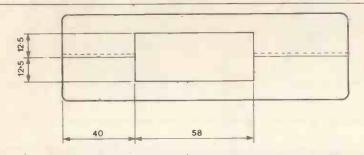
Figure 4. Battery box aperture. The cut-outs must be made in the top moulding end with the groove joint and bottom moulding end with the tongue.
