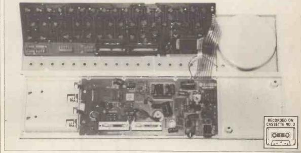
Inside the VL-Tone - the VLSI chip can be seen to the left of the ribbon cable.
