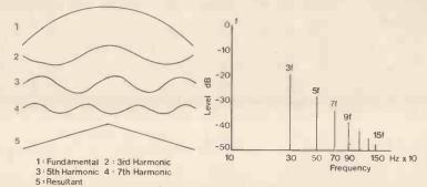
Frequency spectrum of triangle wave, showing harmonic content. Figure 1.
