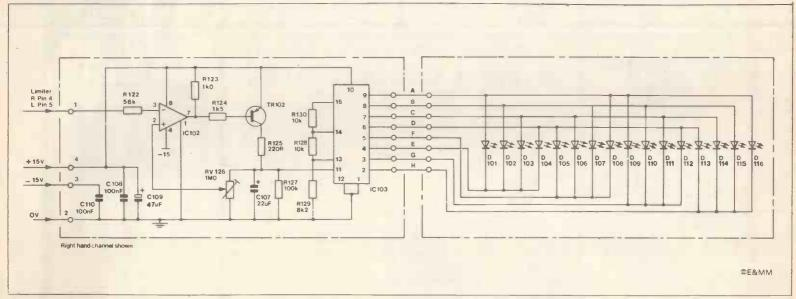
Figure 6. PPM circuit.
