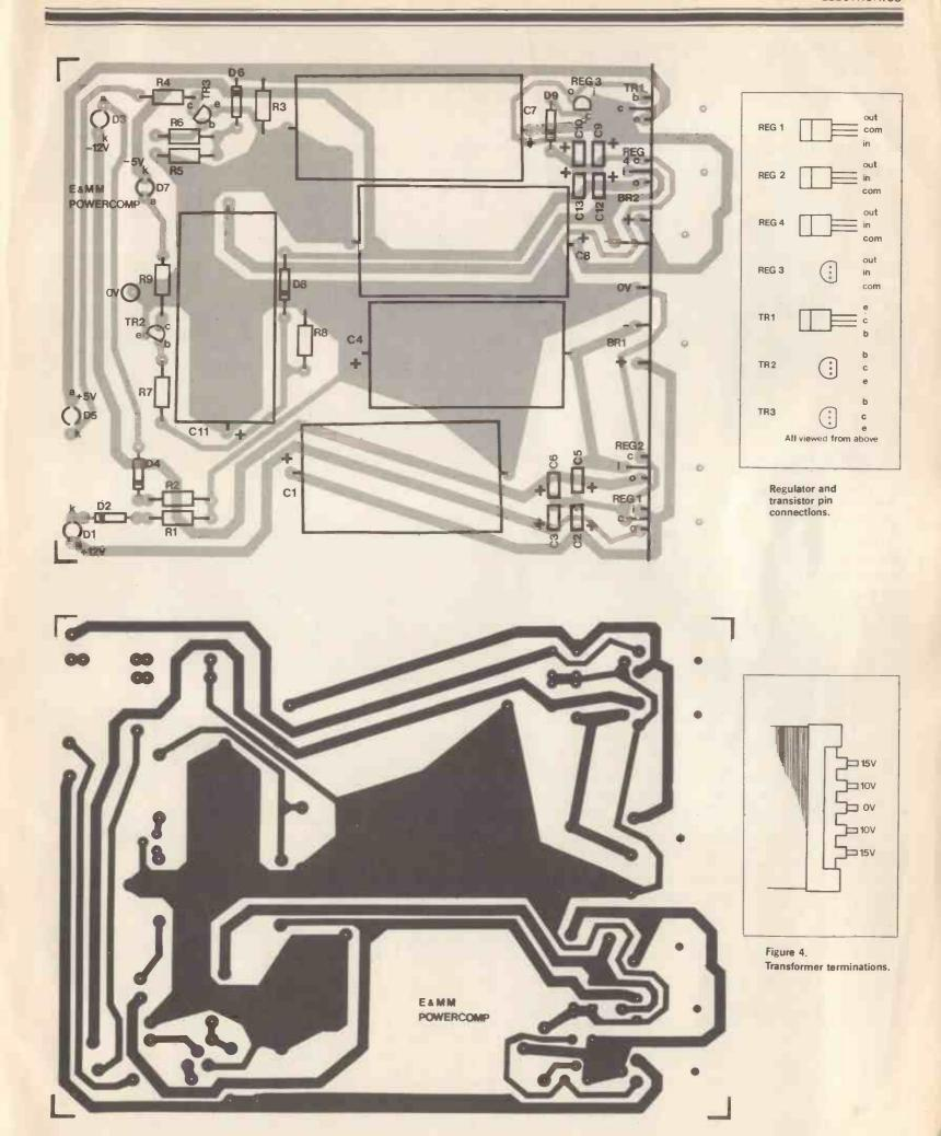
Figure 2. PCB Track and component layouts.
