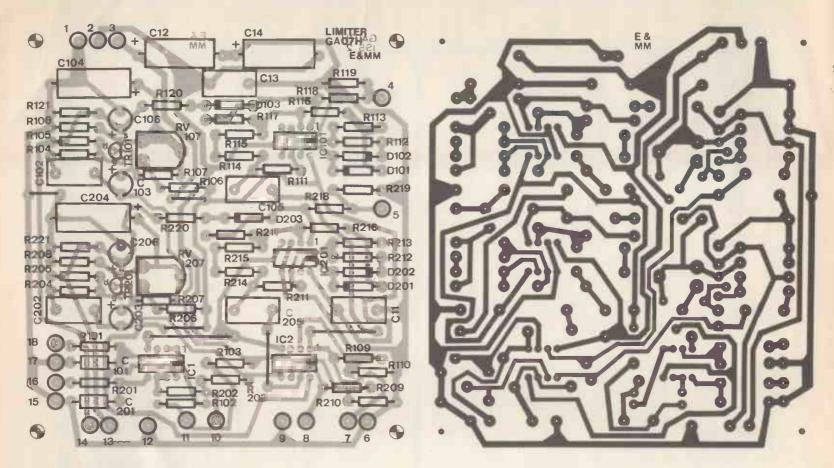
Figure 5. Limiter component overlay and PCB.
