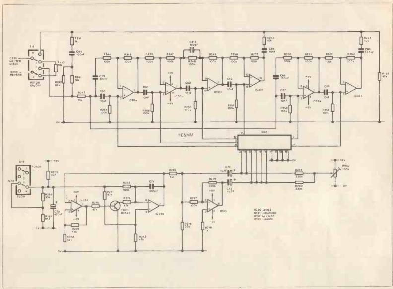
Figure 45. Circuit diagram of the rotor unit.
