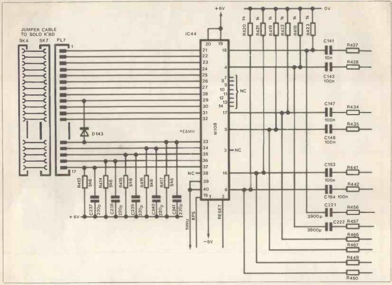
Figure 48. Amended upper manual M108 circuit.
