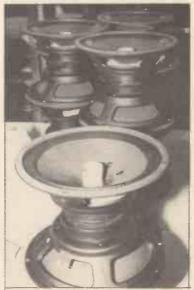
Loudspeaker prior to voice coil insertion.
