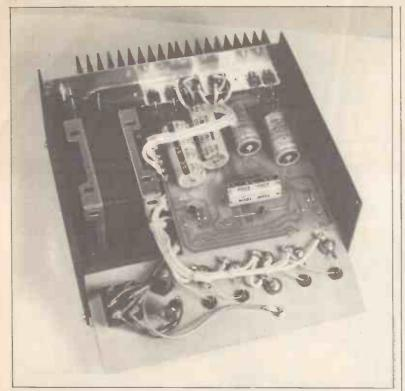
Completed power supply showing internal layout.
