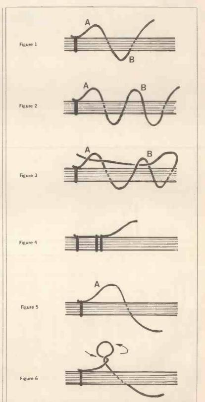
by the addition of a simple whip at the beginning and end of the loom. Again the process of making a whip is simple and straightforward but the results can be very pleasing and professional.
