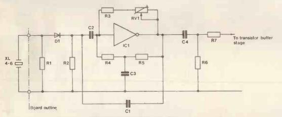
Figure 2(c). Circuit for lower-range drums.
