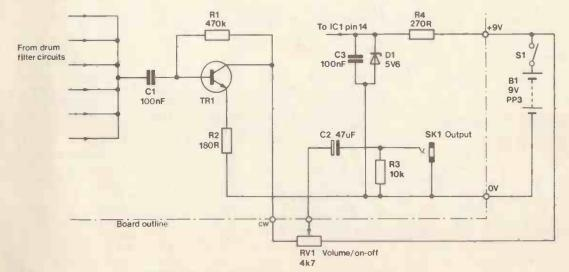
Figure 2(e). Circuit of transistor buffer stage and supply wiring.
