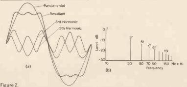
(a) Synthesis of square wave from sine waves. (b) harmonic composition of square wave
