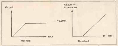
Figure 2. Ideal limiter characteristics
