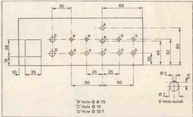
Figure 3(b). Drilling and cutting of front panel.
