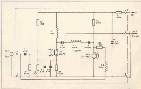
Figure 2. Car aerial booster: circuit diagram.
