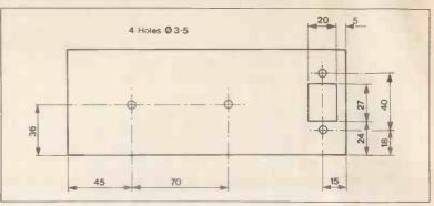
Figure 3(a). Drilling and cutting of back panel.
