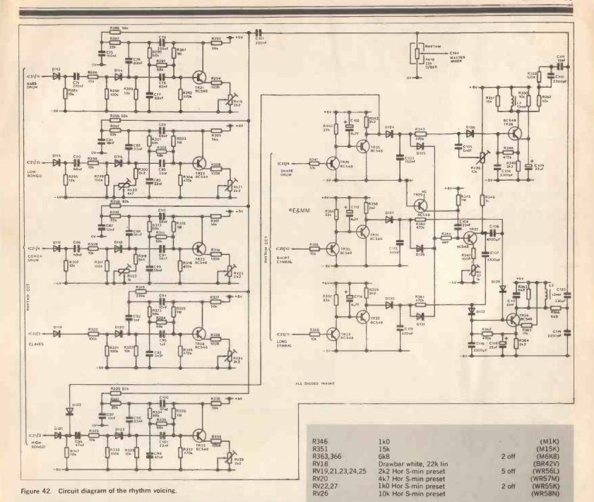
Figure 42. Circuit diagram of the rhythm voicing.
