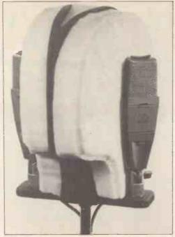
Figure 4. Omni mics baffled from each other for 'dummy head' binaural. Sennheiser MKE203 Electret Capacitor (left) and AKG C414 Capacitor set to omni.
