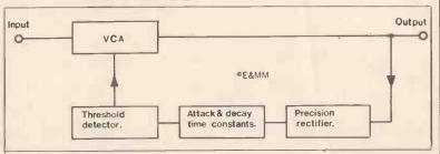
Figure 3. Limiter block diagram.
