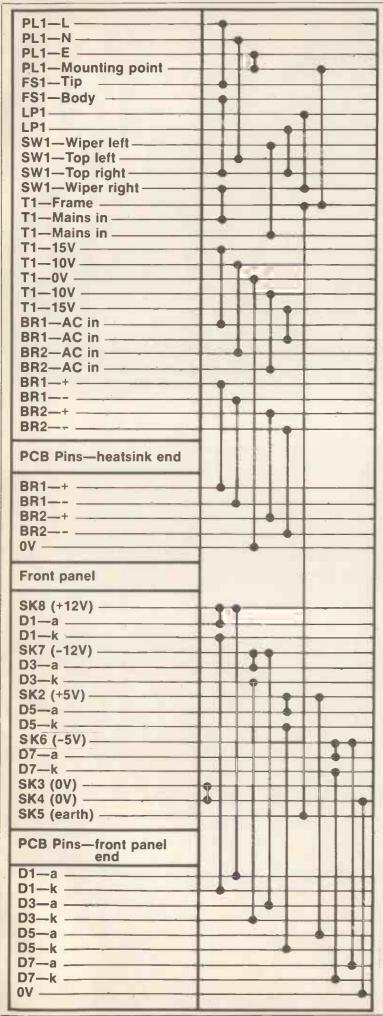
Figure 5. Pianola wiring diagram.
