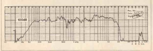
Response chart for Studio 12L & HF250 Crossover HPX4 taken at 1 watt/1 metre in the anechoic chamber. (The dip in response at 600kHz is due to the very small 1½ cu. ft. cabinet used in the test.)
