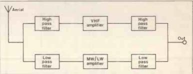
Figure 1. Block diagram of the car aerial booster.
