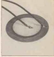
Soldering to the piezo transducers.
