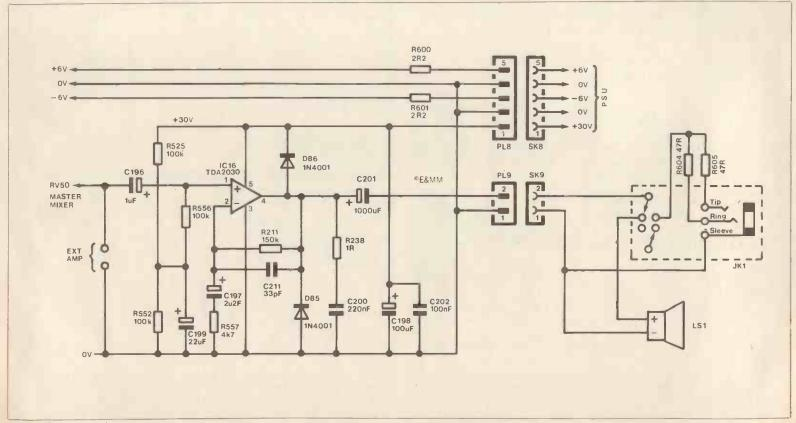
Figure 46. Circuit diagram of the power amp.
