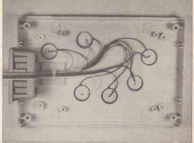
Wiring of the piezo transducers.
