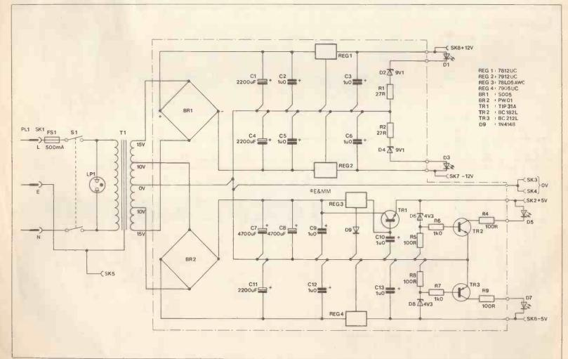
Figure 1. The power supply circuit.
