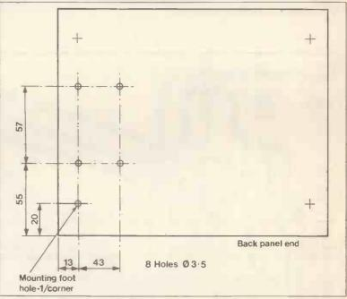
Figure 3(c). Drilling of base plate.
