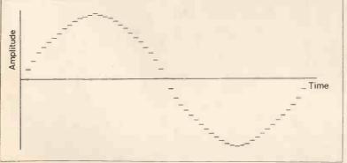
Figure 1. Stair-step sine wave from D/A converter.
