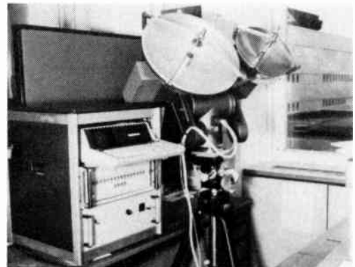
Fig. 13. Ka and W band radiometer imaging system
