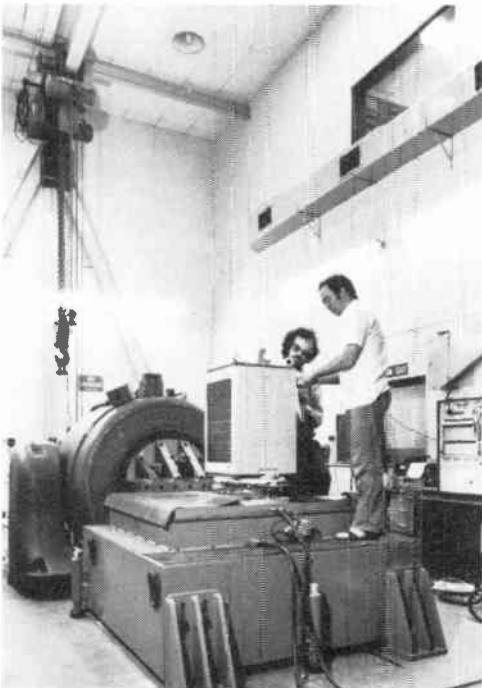
(b) Flight acceptance vibration tests at British Aerospace, Stevenage.
