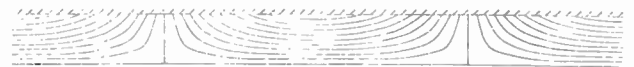
Fig. 10. Magnetization stream function, U_m , for the case when r_m = 0 when in contact with the head.
