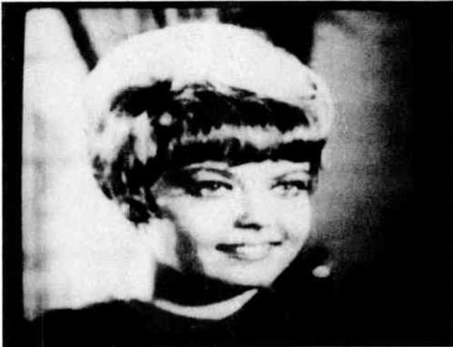
Fig. 9. Recovered picture of the 'Girl' image of Fig. 1 obtained with e.d.l.m.-a.c.s. having k_1 = 1.02 \times 10^6 , k_2 = 32 \times 10^3 , and a n.m.s.e. = 0.107%.
