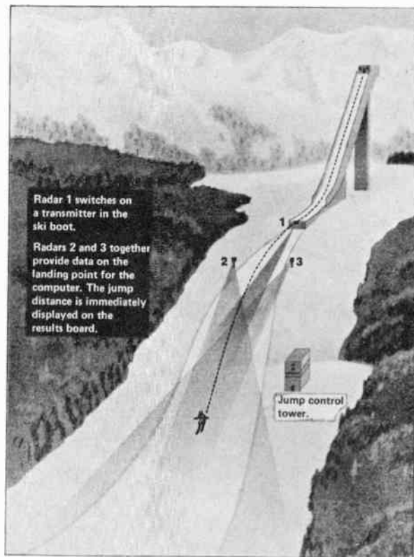
Fig. 9. Sketch of the measurement arrangements at a ski-jumping site. (From U. Pramann. 15 )
