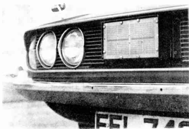
Fig. 3. 0.9 cm f.m.c.w. radar head unit mounted on vehicle (radome removed).
