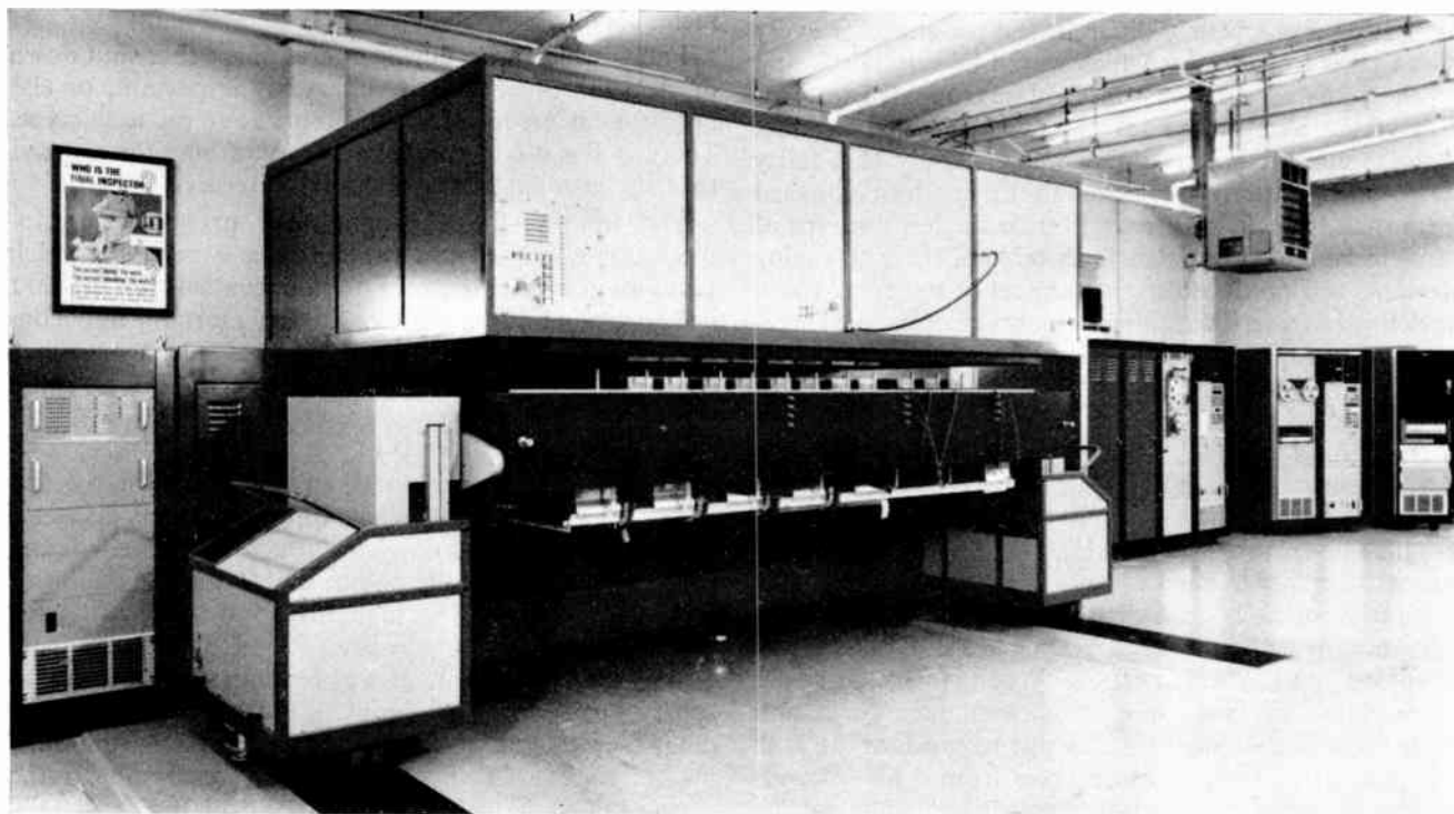
Fig. 6. Overall view of the analyser, computer, and test fixture, showing a TXE 4 rack loaded into a transporter in position for testing.
