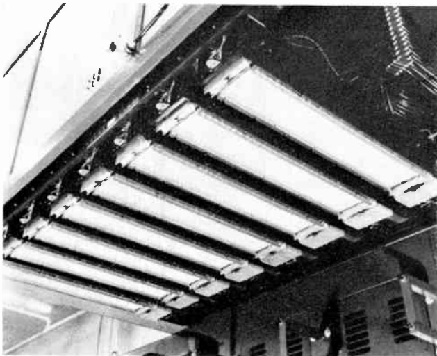
Fig. 5. The 8 test access heads of the analyser test fixture, viewed from below. These accept the plug blades at the top of the boards in Fig. 4.
