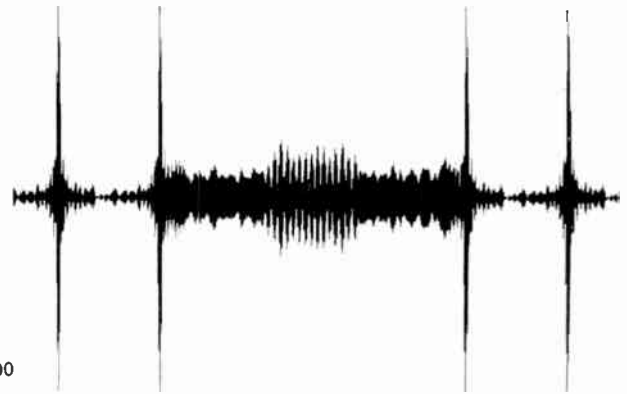
Fig. 6. Output of simulated d.m.t. pulse-compression filter using a 600-stage shift register for a --110011-- data pattern.
