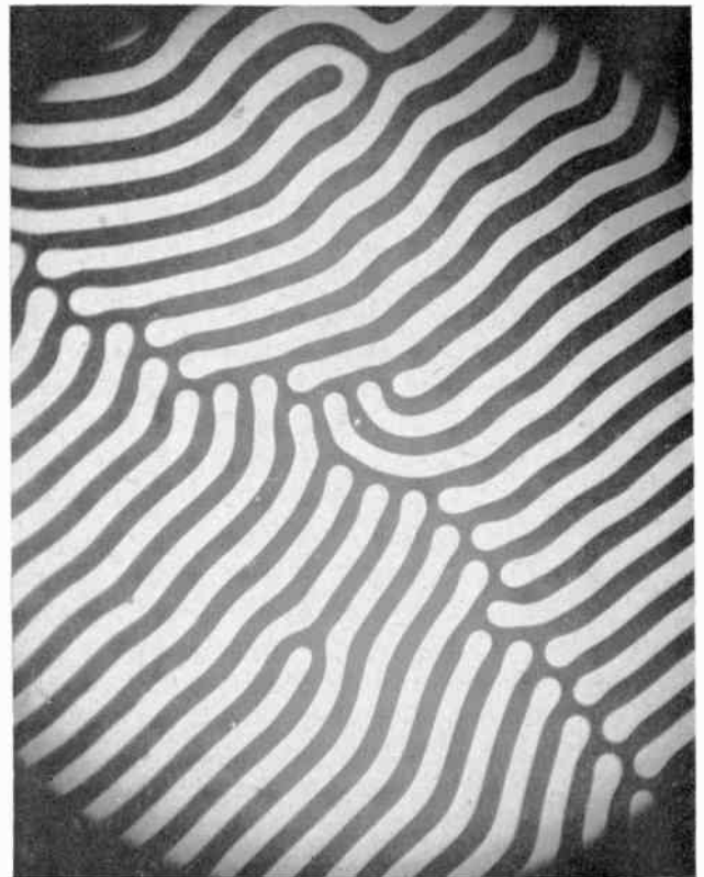
Fig. 10. The path left by a magnetic wire probe demonstrates the cutting of domains.
