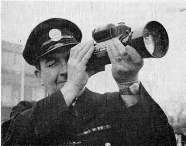
Fig. 6. PPE Lolite direct viewing system. This device has a 20° field of view and the range characteristics shown in Fig. 2.
