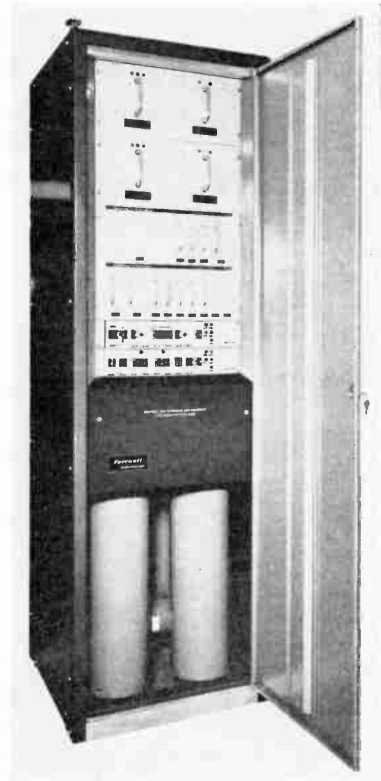
Fig. 4. Typical duplicated multiplex and microwave link terminal.
