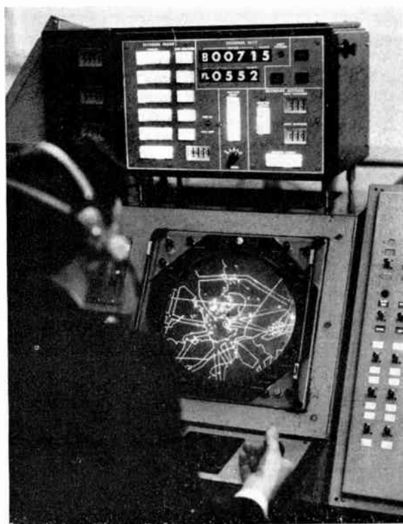
Fig. 13. Prototype model of operator's S.S.R. decoder control unit. The operator has actively decoded a reply on mode B. The code is 0071 (high accuracy is indicated by validity = 5). The altitude is 5500 ft. (Poor accuracy is indicated by validity = 2. The operator would repeat this decoding until validity = 4 at least.)
