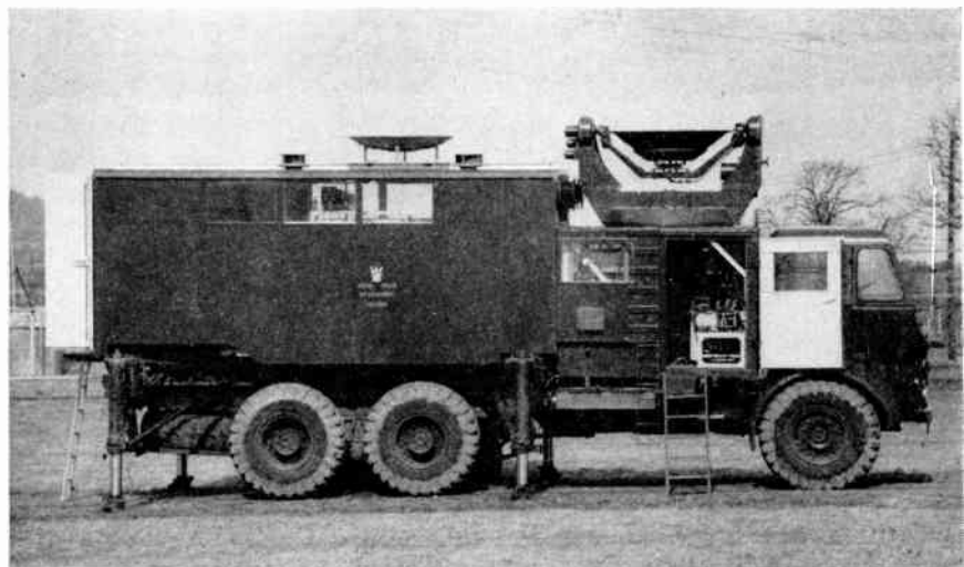
Fig. 7. A mobile Doppler radar, constructed at the Royal Radar Establishment, Great Malvern.
