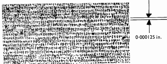
Fig. 7(a). Recording by selective erasure: 32 000 000 bits/square inch.
