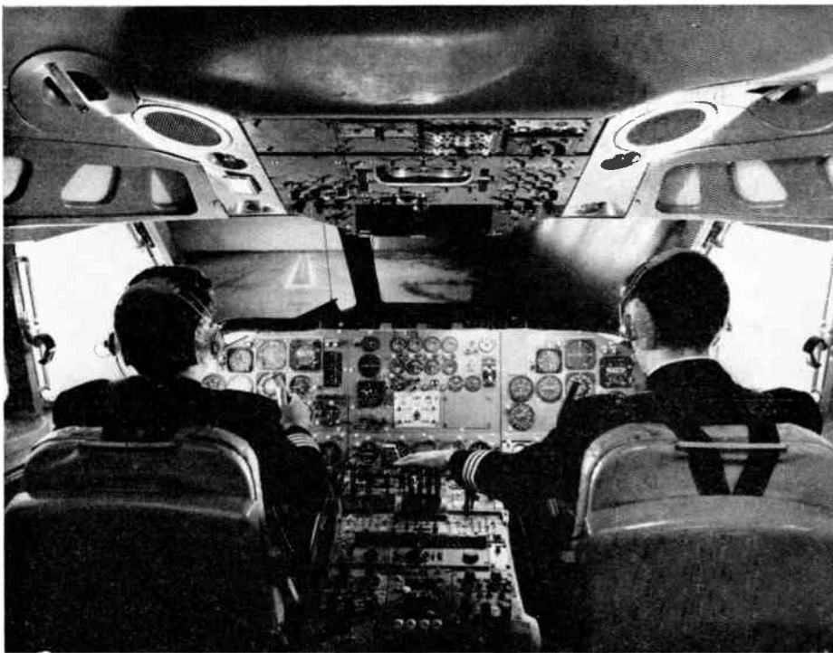
Fig. 13. The Redifon VC10 simulator colour visual system supplied to B.O.A.C. Pilot's-eye view from the flight deck during a simulated approach and landing.
