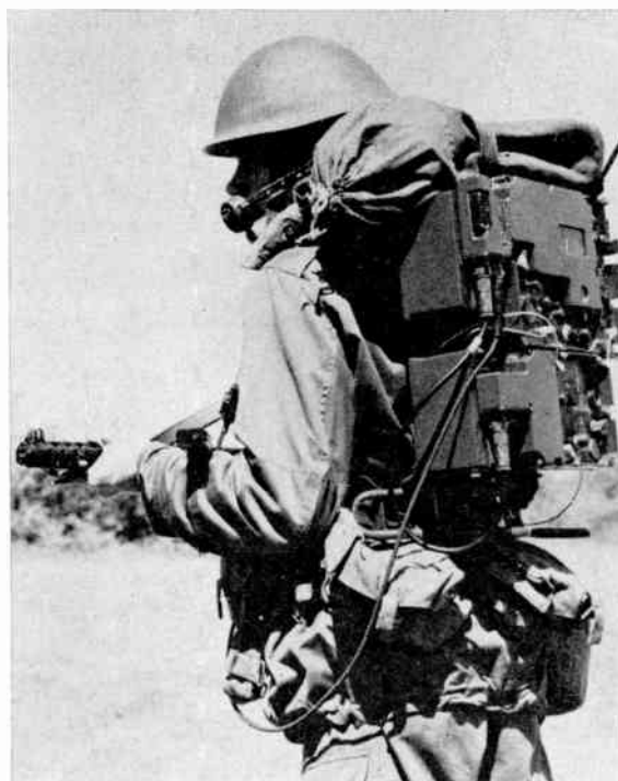
Fig. 9. Station Radio A13 (1964). A modern h.f. manpack transmitter-receiver.
