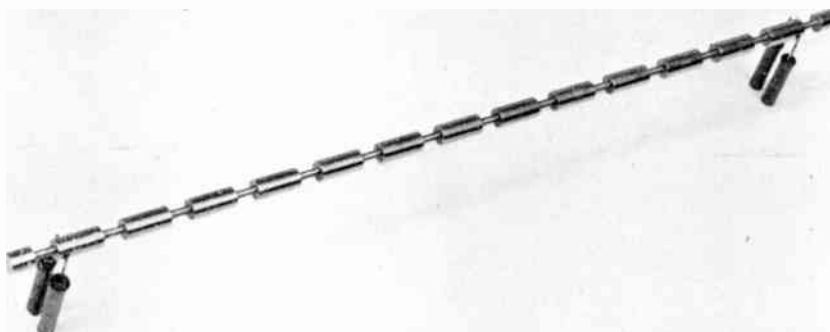
Fig. 1. Torsional-mode single-sideband filter made by turning necks in a rod (with ferrite transducers).
