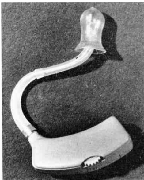
Fig. 11. Hearing aid designed to be worn behind the ear. Size 1.4 in \times 0.5 in \times 0.5 in.
