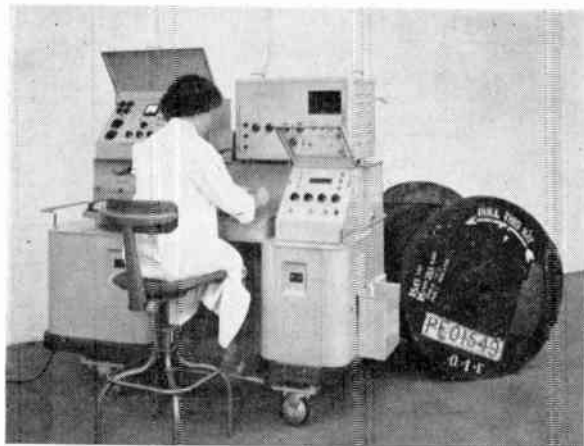
Fig. 10. A final stage cable test set in use.
