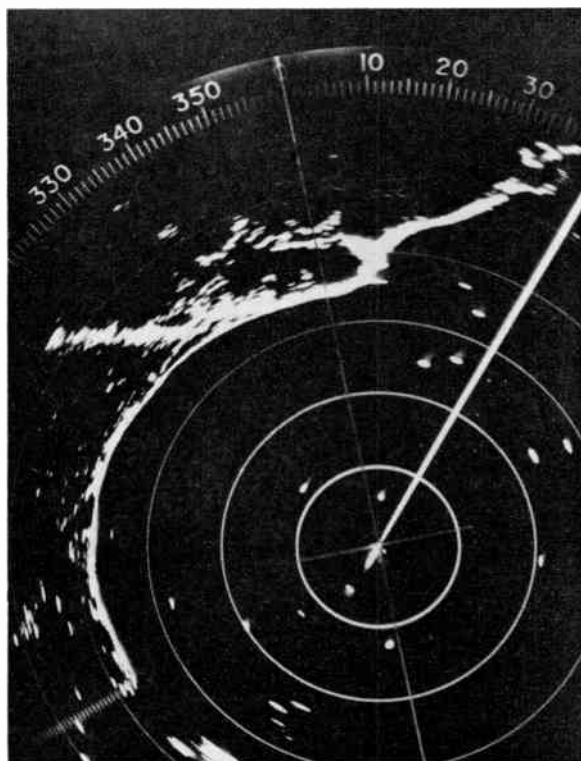
Fig. 8. Radar p.p.i. showing racon signal.
