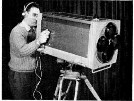
Fig. 15. The E.M.I. colour camera as demonstrated before the Institution on 17th December 1958.
