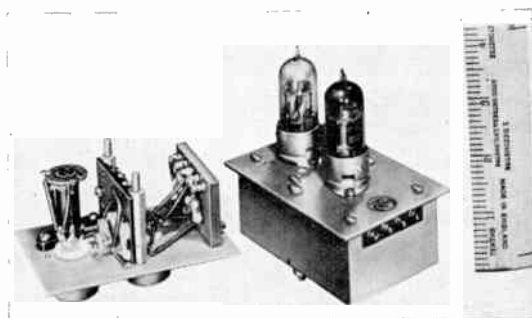
Fig. 6. Crystal oscillator: thermally-compensated type.
