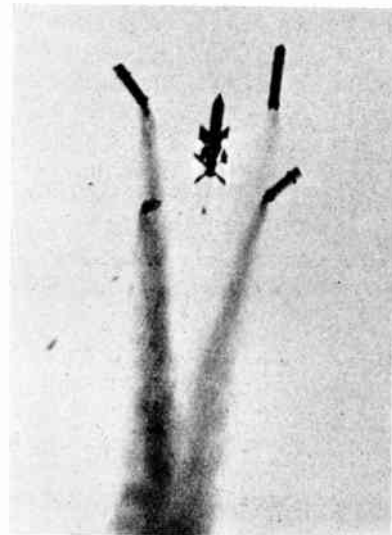
Fig. 1. Experimental firing of guided weapon "Sea Slug". The photograph shows the jettisoning of the four booster rockets. (By courtesy of Armstrong Whitworth Aircraft.)
