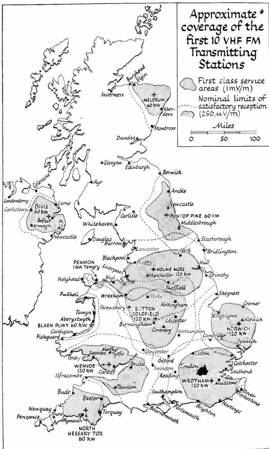
Fig. 1.—This map illustrates the coverage to be expected from the ten stations to be erected in Stage I of the V.H.F. Plan. The station at Penmon is a temporary expedient pending the erection of a three-transmitter station in Stage II of the Plan.
