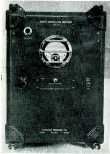
Fig. 13.—Indicator unit for ring dynamometer.
