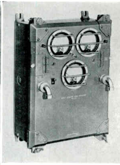
Fig. 14. — Double indicator, for measuring the prestressing in concrete re-inforcements.
