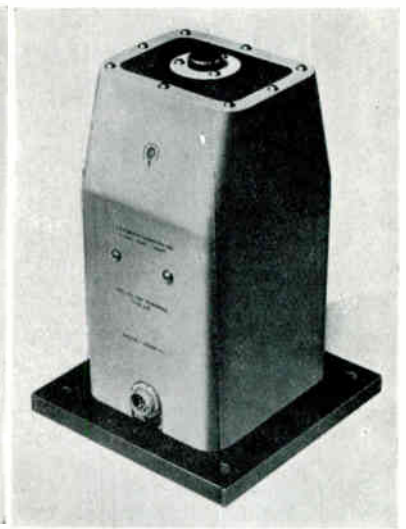
Fig. 15.—Converter for using tension dynamometers in compression.
