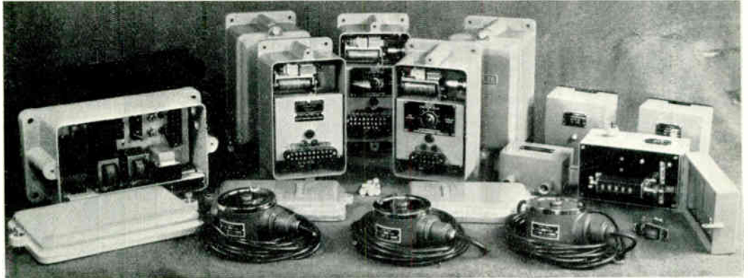
Fig. 3.—Load cells and associated magnetic amplifiers.
