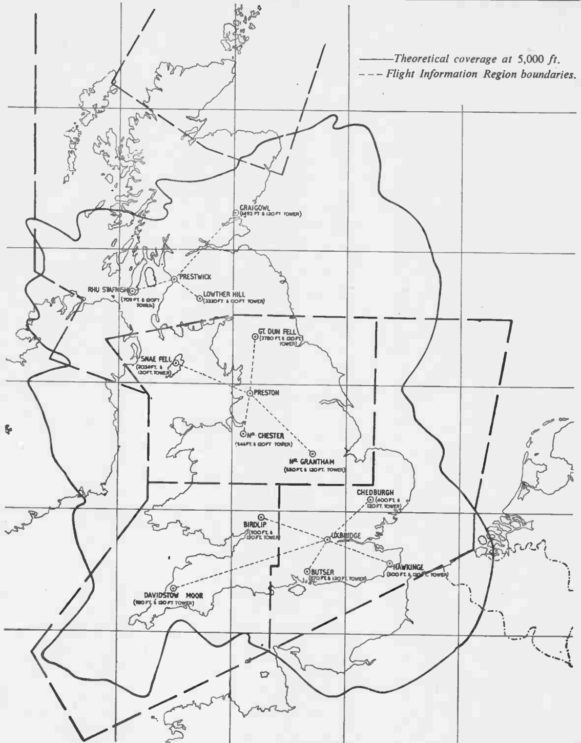
Fig. 5.—Layout of M.C.A. V.H.F. area coverage network.
