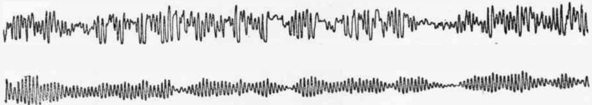
Fig. 6. This figure gives an indication of the performance of the resonant amplifier. Channel I shows a complex Waveform, and Chan. II the 8 c/s component obtained from a monitoring point on the output of V_2 .
