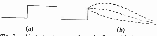
Fig. 2.—Unit step impressed on the first grid gives these fundamentally possible responses. They all tend to zero.
