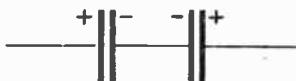
Fig. 13a.—Two electrolytic condensers connected "back to back" for operation as a single reversible or non-polarised unit.
