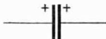
Fig. 13b. — Equivalent effect produced by winding the two positive foils in one unit and omitting negative foils.
