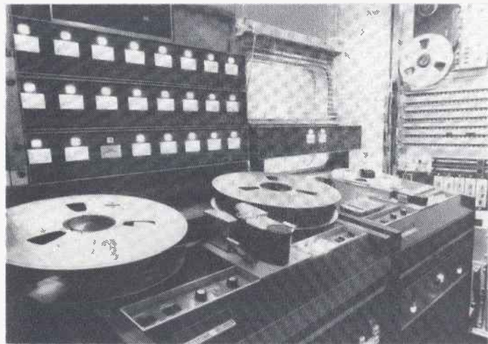
Centrepieces of the recording studio are these two 3M Mincom M79 recorders: the 24-track unit (left) and a Half-track stereo version of the M79 for mix-down purposes.
