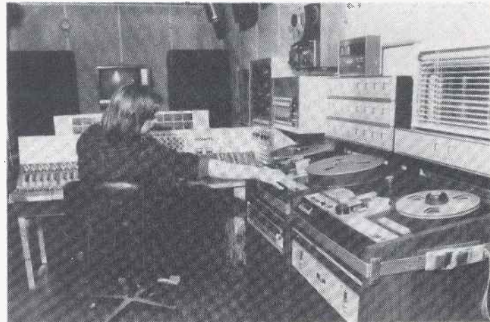
Engineer Mick McKenna at the Helios desk control system which provides 32 inputs and has facilities for 60 microphone lines. Altec 604/8G loudspeakers provide monitoring facilities.
