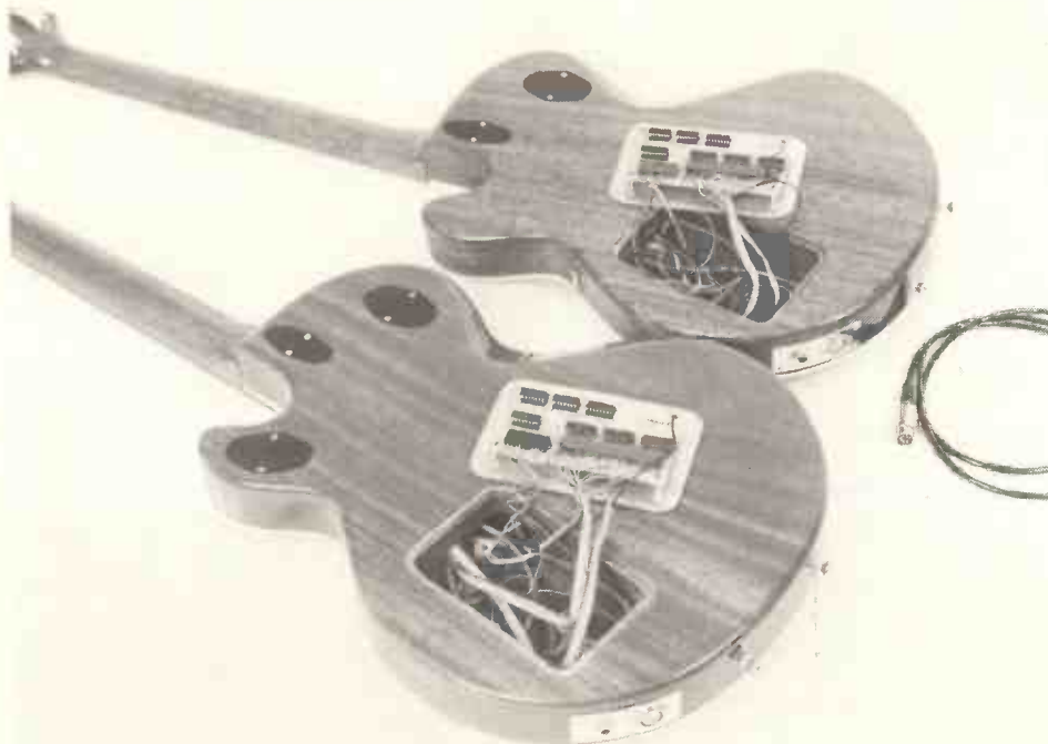
The internal circuitry of the Hagstrom 'Patch 2000' synthesizer guitar showing the bass (below) and lead version (above)
