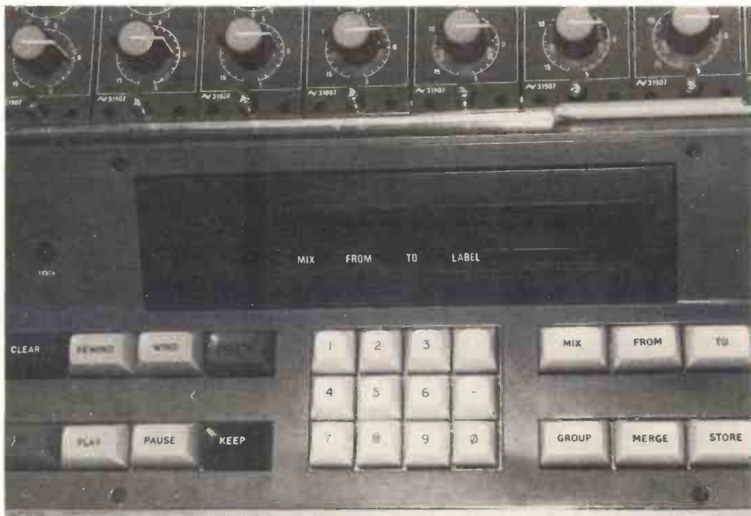
▲ Close up of the automatic faders and ▼ the computerised 'memory bank'.
