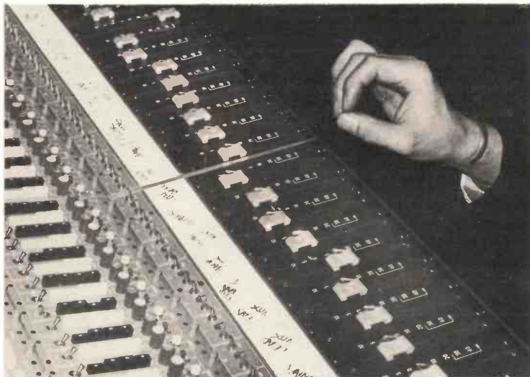
▲ Close up of the automatic faders and ▼ the computerised 'memory bank'.
