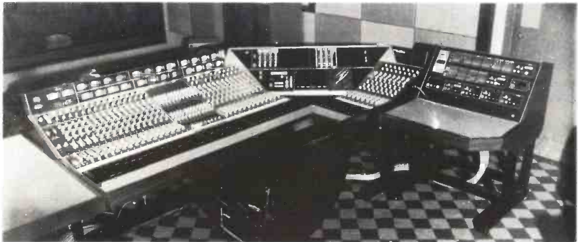
A 32 channel, 24 track recording and re-mixing console supplied to Island Records, London. The console has parametric channel equalisers, peak metering, programmeable "cut" facilities and a purpose built tape machine remote console.
