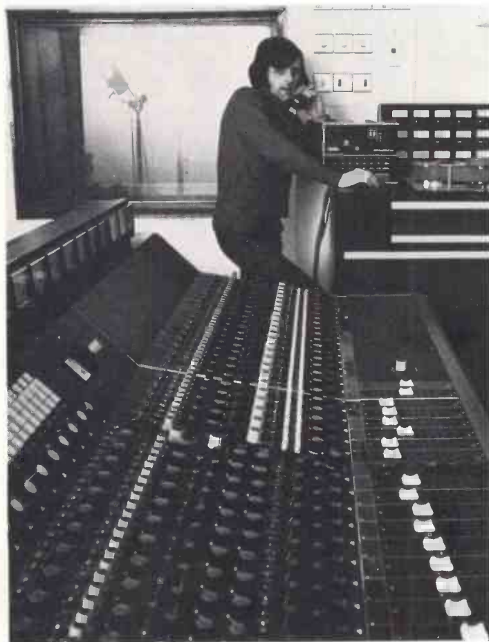
Barry Ainsworth in Sarm's Main Control Room. The Triad 24-track desk is in the foreground and the MCI recorder behind
