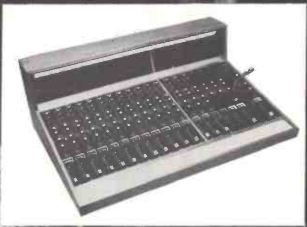
R.S.D. Mk. III MIXER. Modular microphone channels, any number as required. Two master output modules. One foldback output module (for storage monitors). One echo master module. One internal monitor module. Housed in teak finished case. Supplied in wooden travelling case. Mic. channel module controls: Signal input attenuator. Mic. channel gain. Echo gain. Switch for Echo 1 or Echo 2 or Echo 3. Treble lift and cut (-15db @ 15KHz). Bass lift and cut (switchable to operate on 50, 100, or 200 Hz) (-15db). Presence (middle) lift (switchable to operate at 0.4, 1.0, 2.2, 3.5 or 7.0 KHz) 12db. Pan left and right. Channel on/off and internal monitor switch. Meter. Main fader (sliding potentiometer). Noise figures: - Relative input noise: Better than -125dbm. Quiescent S/N Ratio: All faders down to 80dbm. Average setting for use: S/N Ratio 75dbm.
