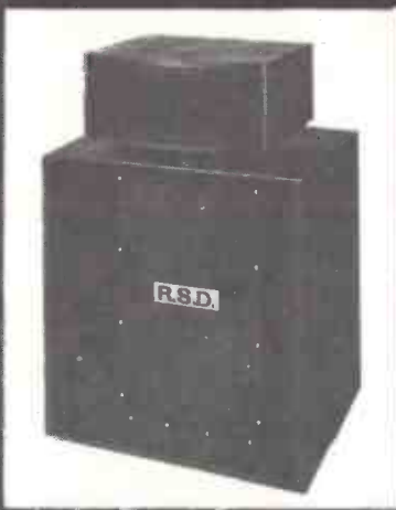
R.S.D. 215A-Type. Horn loaded. Bass cabinet. Frequency response 30-20000 Hz. Power Rating 300 Watts R.M.S. 1000 Watts Peak to Peak. SPL not less than 130db at 50' from source sweep 100 Hz 1600 H3. R.S.D. 215AR-Type. Folded Horn bass cabinet. Response: 30 Hz to 1000 Hz. Power Rating 300 Watts R.M.S. 1000 Watts Peak to Peak. SPL not less than 125db on 50' sweep at 600 Hz.
