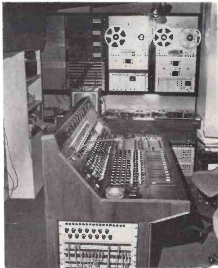
The control room: in the foreground is the Electrosonic desk and behind are the Leever-Rich/Richardson recording machines.
