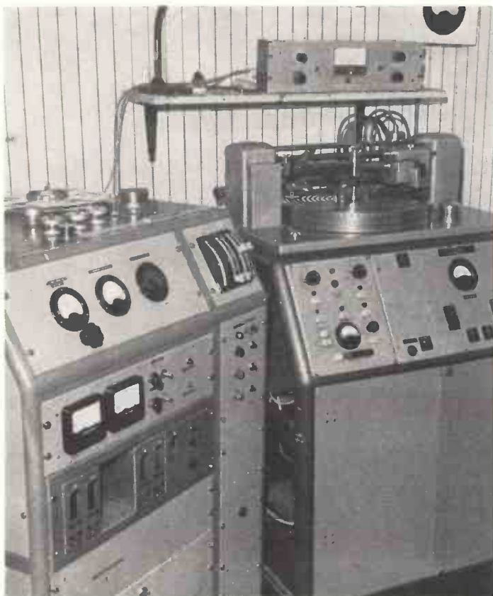
The cutting room facilities with the Lyrec mono cutter and Ortofon cutting console
