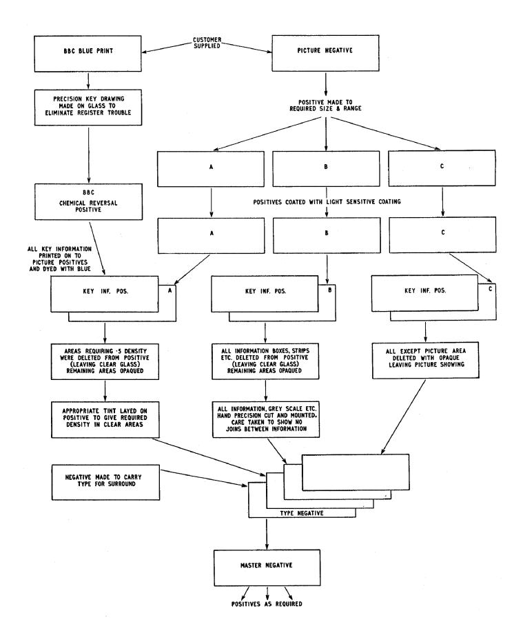
Fig. 8 — Manufacturing schematic for Test Card No. 51
