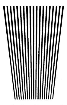
Fig. 4 — A typical frequency wedge
