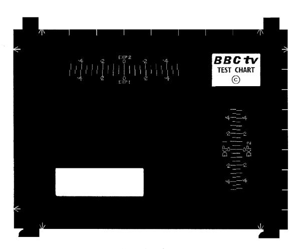
Fig. 11 — Hop and weave tests
