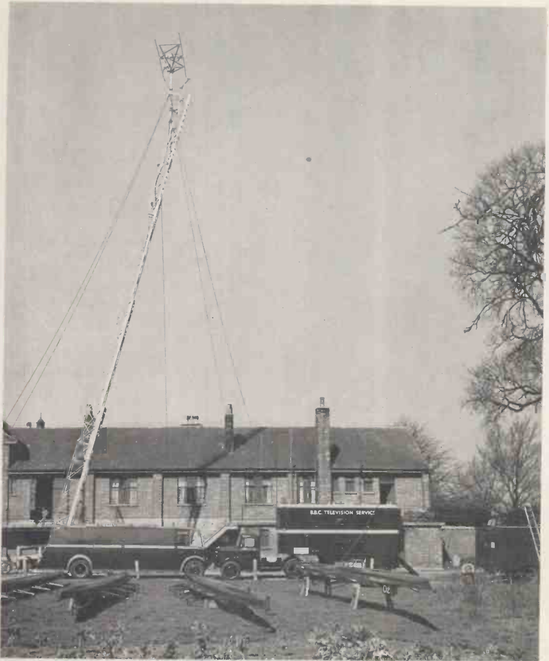
THE BOAT RACE 1949: A mobile aerial, mounted on a fire escape, near Chiswick Bridge.
