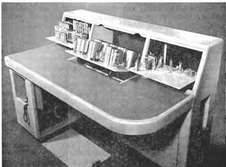
Fig. 2.11. Studio control desk Type A, Mark V. The top photograph shows a general view of the control desk and the lower photograph shows the panels swung forward for inspection and maintenance with the side panel of the pedestal removed
