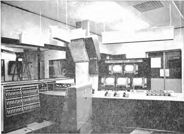
Fig. 3.11. A lighting and vision control room, with lighting console shown on left
