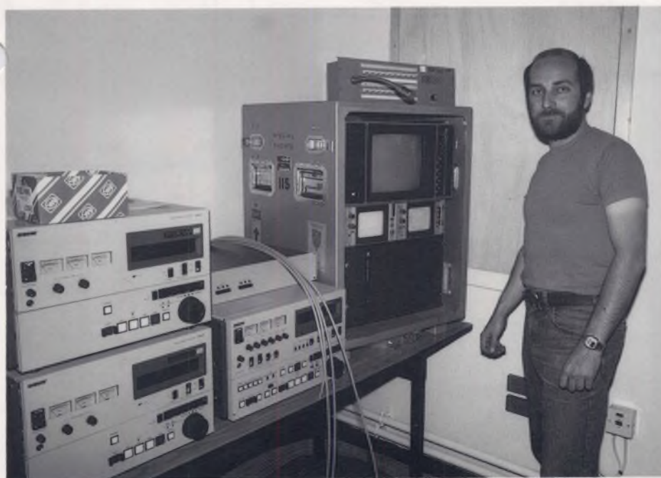
Canadian technician installer Graham Campbell alongside the Betacam half-inch VT machines arranged for editing. Note the equipment built inside the flight package.
