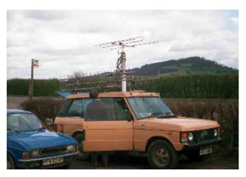
verify the predicted service area. (Above Alun Maddocks is checking the antenna on the borrowed Range Rover) Unfortunately the new transmitters caused interference to listeners of the Pontypool VHF relay station and so the service was temporarily closed down after a week. The problem was eventually cured by changing the frequency of the smaller Pontypool relay.
