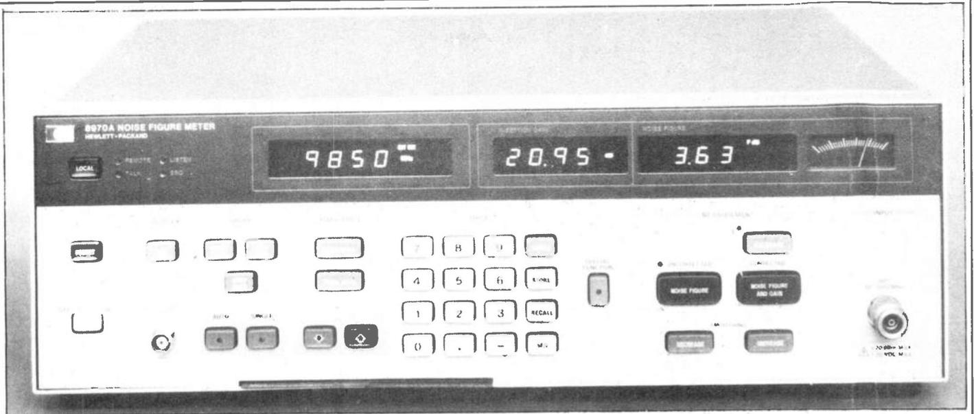
Above: the Hewlett Packard 8970A noise figure meter, used by Angus McKenzie for last month's review of preamps, converters and transverters.
