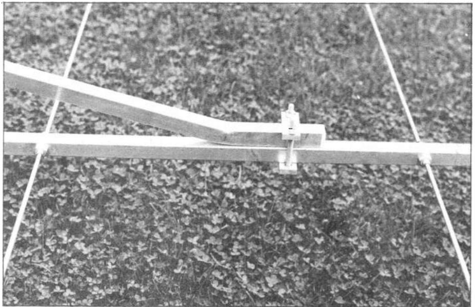
Supporting brace bolted to boom with clamp
