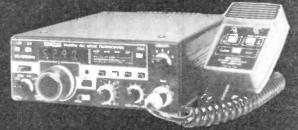
The recently introduced IC-290H has proved so popular that we have decided to concentrate on this (25W) model 2m multimode. With its bright green display. 5 memories, scan facilities on either memories or the whole band, tone-call button on the microphone and instant listen input for repeaters, this little box really is a beauty. The 70cm version, the IC-490E has similar features (although the output is only 10W in this case)
