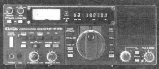
The R-70 covers all modes (when the FM option is included), and uses 2 CPU-driven VFO's for split frequency working, and has 3 IF frequencies: 70MHz, 9MHz and 455KHz, and a dynamic range of 100dB. It has a built-in mains supply.
