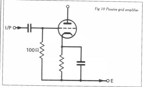
author used it for a while and found it quite effective. This design was only possible because of the internal construction of the 6J6 and it is doubtful whether it could be applied successfully to other types of valves.
