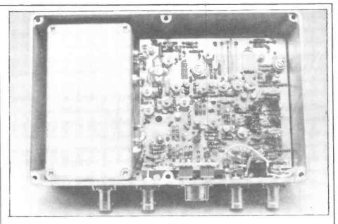
Above: Microwave modules 432MHz transverter. Bottom of page: Lunar preamplifier.
