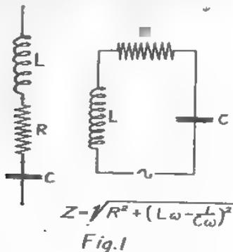
connected in series (see Fig. 1), is given by the following relation (see Fig. 1).
