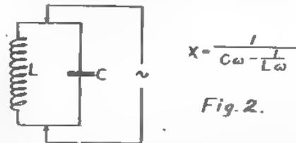
If, however, the emf is applied in parallel to the inductance and capacity (see Fig. 2), an entirely different value of impedance is found. In this case
