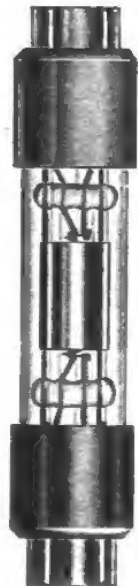
RAC-3 Audions. The first Universal Audion for reception and amplification.
